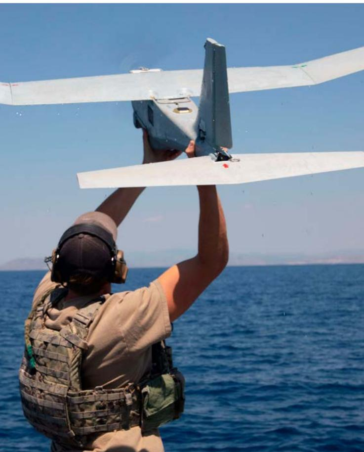
A U.S. Navy Special Warfare Combatant-Craft Crewman assigned to Naval Special Warfare deploys the Puma All Environment Unmanned Aircraft System during a training mission with Hellenic Navy special operators from the Underwater Demolition Command (DYK) in the Aegean Sea. Source: U.S. Army photo by Sgt. Aven Santiago
