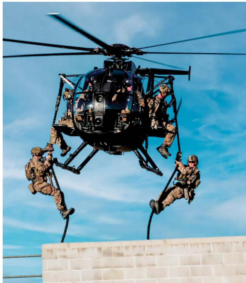
Rangers deploying from an MH-6M – a light utility helicopter modified to externally transport several combat troops – via fast rope. Source: U.S. Army Private First Class Gabriel Segura
