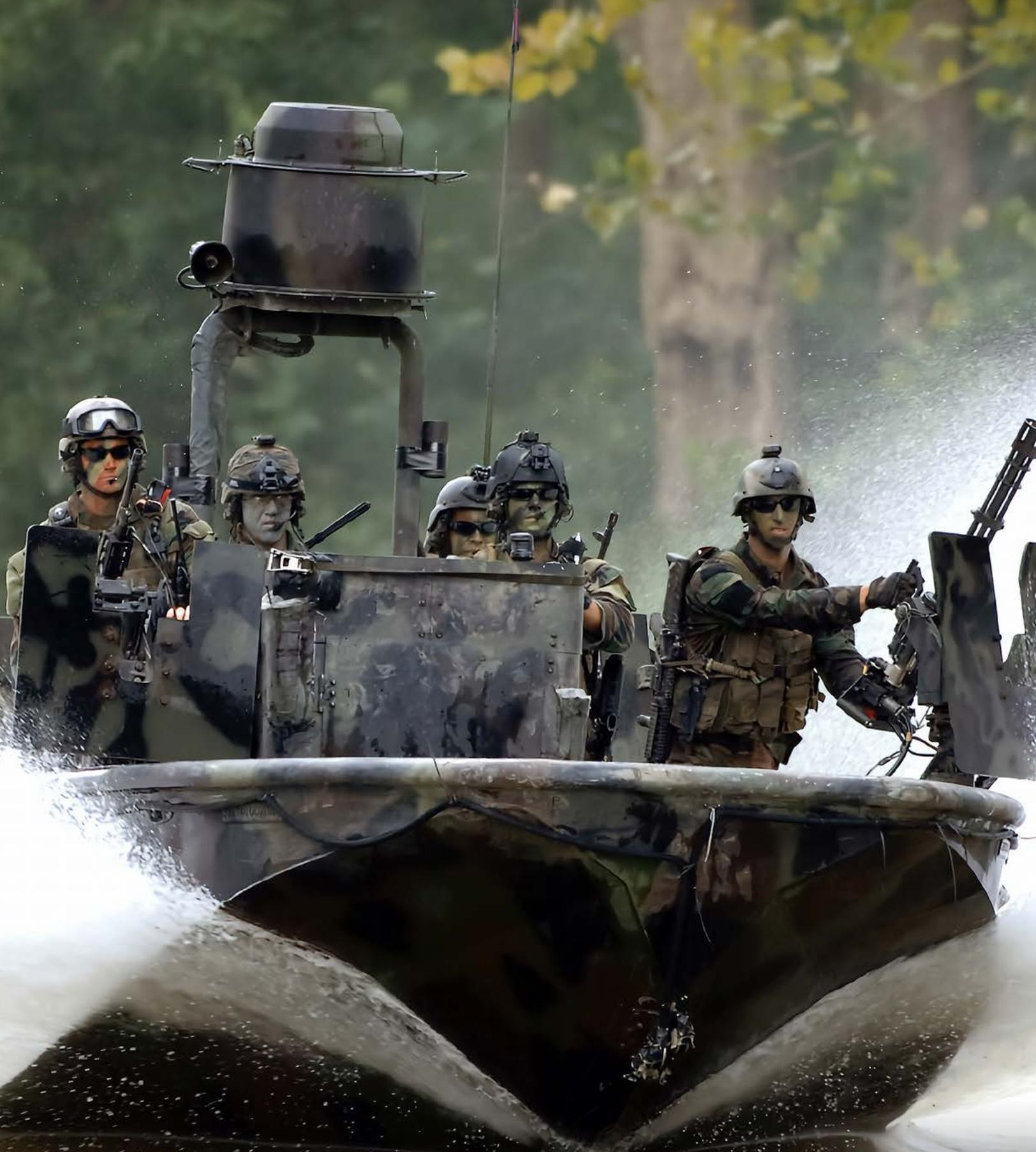
Special Warfare Combat Crewmen transit the Salt River in northern Kentucky during pre-deployment, live-fire training, employing the Special Operations Craft Riverine, which is specifically designed for the clandestine insertion and extraction of U.S. Navy SEALs and other special operations forces along shallow waterways and open water environments. Source: U.S. Navy photo by Mass Communication Specialist 2nd Class Jayme Pastoric
