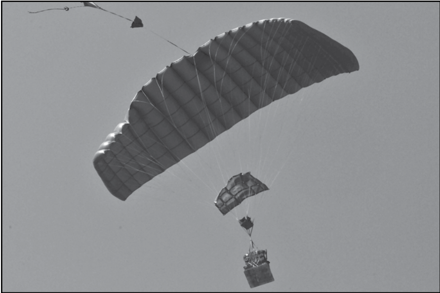
Figure 2. A JPADS guides itself to the ground following its drop from a C-130 aircraft at Normandy Drop Zone in Fort Bragg, North Carolina. Source: U.S. Army photo by Sergeant Amanda Tucker
